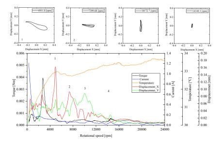
Figure 4 The characteristics of torque, electric current, temperature and displacement as a function of rotational speed recorded during run-up No. 1
