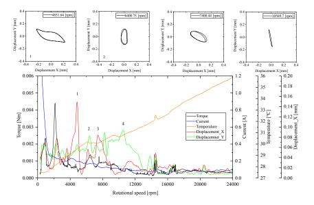
Figure 5 Torque, electric current, temperature and displacement characteristics as a function of rotational speed recorded during run-up No. 2  $\,$
