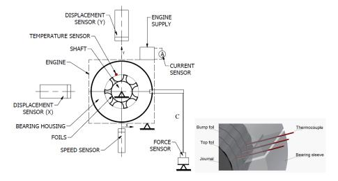
Figure 1 On the left: Test stand for experimental determination of the lift-off speed of foil bearings. On the right: Arrangement of thermocouples [11]
