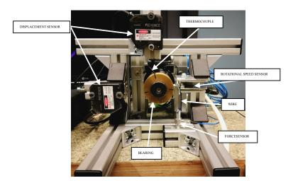
Figure 2 Photo of the test stand for experimental determination of the lift-off speed of foil bearings
